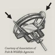
**Open the Trap:** If possible, pull the trap chain tight from the anchor point and put the trap flat on the ground. To open the trap, push down using your hands or feet on the levers located at either end of the jaws (see arrows in the diagram). This will release tension on the jaws and allow you to remove the dog's foot.
